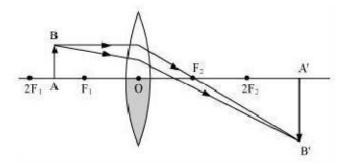
**Question 21:** An object 5 cm in length is held 25 cm away from a converging lens of focal length 10 cm. Draw the ray diagram and find the position, size and the nature of the image formed.
